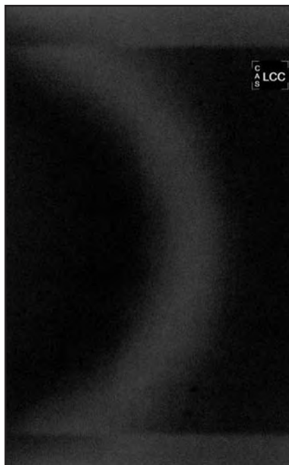
FIGURE 7. Ghosting artifacts can occur when the energy from previous images is not completely removed from the imaging detector following exposure.
